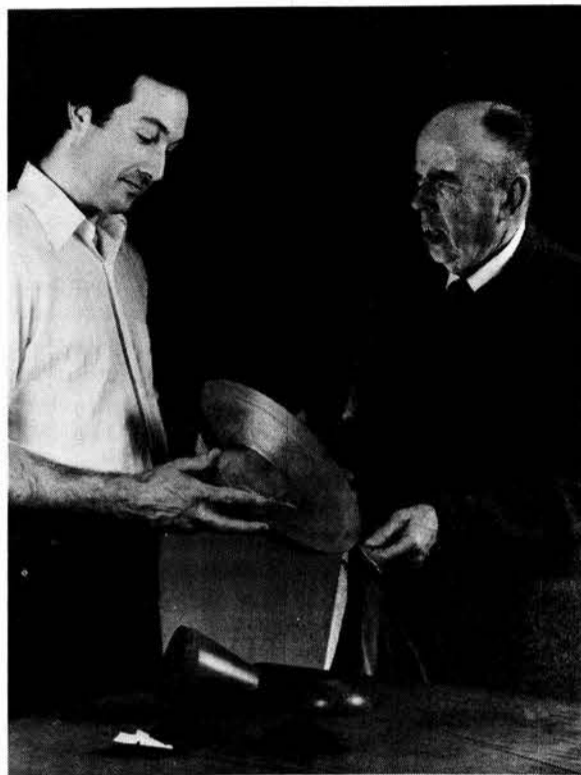
CONCAVE COLLAR was shaped, quite intentionally, with an opening on the (left) side, from molded desiccant foam, as displayed by foam developer Chuck Frost (right) and senior technician Patrick Keifer (both 8315). The new foam acts as both a drying agent and a structural support for electronic components. The tapered cylinder, rounded cap, and other wedge shapes (below) were molded from the same material.
